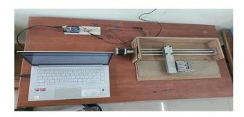
The students under product development club developed a **'Tape Casting Machine'** to make thin ceramic tapes of upto 10micron thickness, to be used as substrates or as electrodes in fuel cells.
