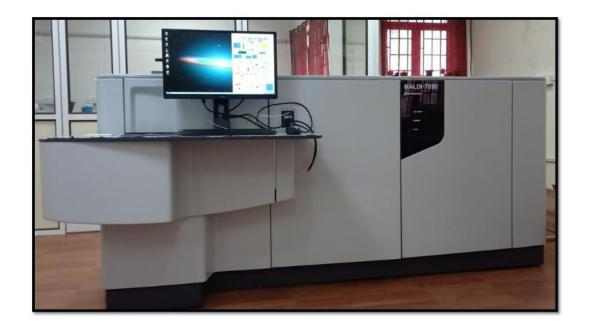
The MALDI-7090<sup>TM</sup> is a state of the art, high-resolution MALDI-TOF/TOF mass-spectrometer and one of the latest in the field of MALDI-TOF mass-spectrometry. The instrument is primarily focused on protein characterization and proteomics. Mascot search engine is used for database searching. Additionally, targeted analysis of other biomolecules is also done. Users are requested to follow the sample submission instructions and provide the necessary details.
